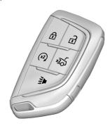
**a**: Press to lock all doors and the fuel door, if equipped. The turn signal indicators may flash and/or the horn may sound on the second press to indicate locking. See *Vehicle*Personalization ⇔ 120.
