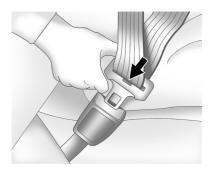
3. Push the latch plate into the buckle until it clicks. Pull up on the latch plate to make sure it is secure.
