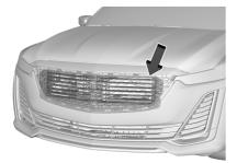
The vehicle may have a shutter system designed to help improve fuel economy. Keep the shutter system clear of debris, snow and ice. If the check engine light is activated, please check to see if the shutter system is clear of debris, snow or ice.
