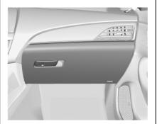
Pull the handle from the side to open the glove box. Close until it latches. Use the vehicle key to lock or unlock.
