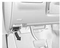
Pull the hood release lever with the symbol. It is on the lower left side of the instrument panel.
