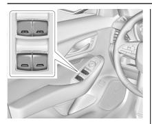
Power windows work when the ignition is on, in ACC/ACCESSORY, or when Retained Accessory Power (RAP) is active. See *Retained Accessory Power (RAP)* ⇒ 212.
