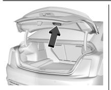
Close the trunk by pulling on the handle. Do not use the handle as a tie-down. Do not press the touch pad while closing the trunk; this will cause the trunk lid to be unlatched.
