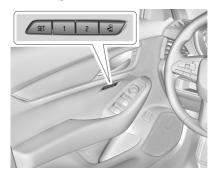
If equipped, memory seats allow two drivers to save and recall their unique seat positions for driving the vehicle, and a shared exit position for getting out of the vehicle. Other feature positions may also be saved, such as power mirrors and power steering wheel, if equipped. Memory positions are linked to remote key 1 or 2 for automatic memory recalls.
