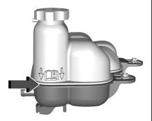
If coolant is visible but the coolant level is not at or above the indicated mark, add a 50/50 mixture of clean drinkable water and DEX-COOL coolant.
