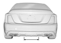
If equipped, the trunk may be opened with a kicking motion under the rear bumper at the location of the projected logo. The remote key must be within 1 m (3 ft).
