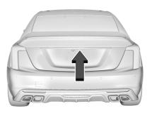
Press the touch pad on the rear of the trunk above the license plate when all doors are unlocked.
