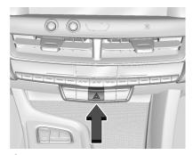
⚠: Press this button to make the front and rear turn signal lamps flash on and off. Release the button for at least one second and press again to turn the flashers off.
