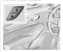
**a**: Press to lock the doors. The indicator light in the switch will illuminate when locked.
