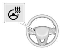
②: If equipped, press to turn the heated steering wheel on or off. An indicator light next to the button displays when the feature is turned on.
