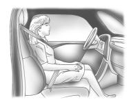
If a person of adult size is sitting in the front outboard passenger seat, but the off indicator is lit, it could be because that person is not sitting properly in the seat or that the child restraint locking feature is engaged. Use the following steps to allow the system to detect that person and enable the front outboard passenger frontal airbag and knee airbag:
